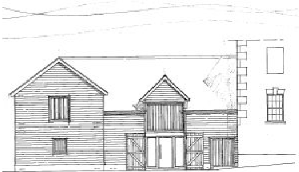
PROPOSED EAST ELEVATION 1:100
